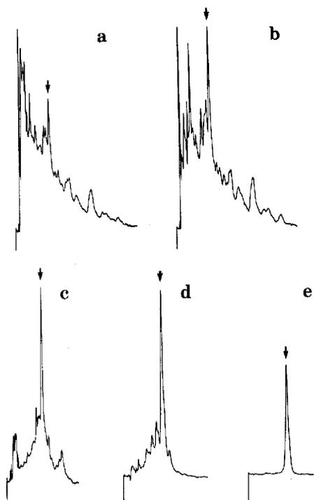
Fig. 2. Analytical high-performance liquid chromatograms of azadirachtin (arrows) recovered after: (a) dichloromethane extraction; (b) silica gel flash chromatography; (c) ODS flash chromatography; (d) silica gel preparative HPLC; (e) phenyl preparative HPLC. Analytical HPLC was performed with a phenyl column (25 × 0.46 cm I.D., 5  $\mu$ m particle size) eluted isocratically with acetonitrile-water (3:7) at 1.0 ml/min.
